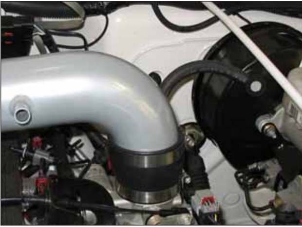
f. Insert the intake pipe into the rubber coupler attached to the throttle body.
