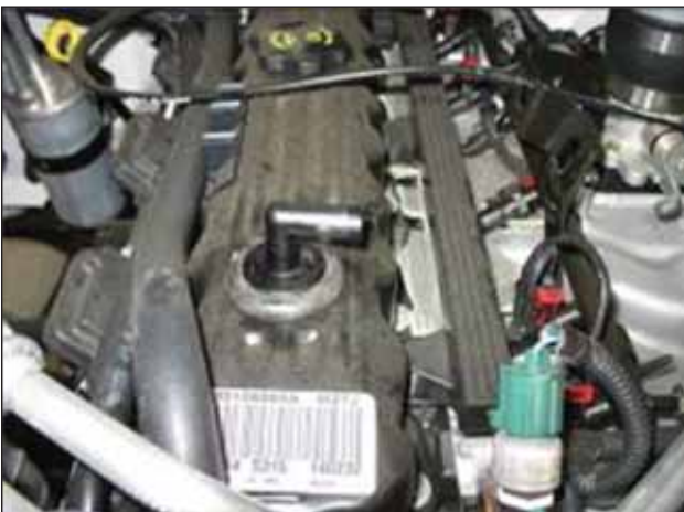
j. Twist the stock nipple carefully until it faces the driver side of the vehicle.
