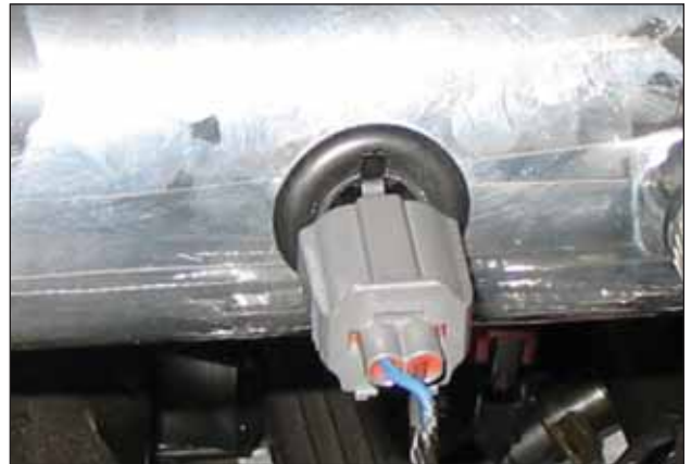
i. 2005-2006 Vehicles: Carefully install the IAT sensor into the intake pipe. 1997-2004 Vehicles: Proceed to the next step.
