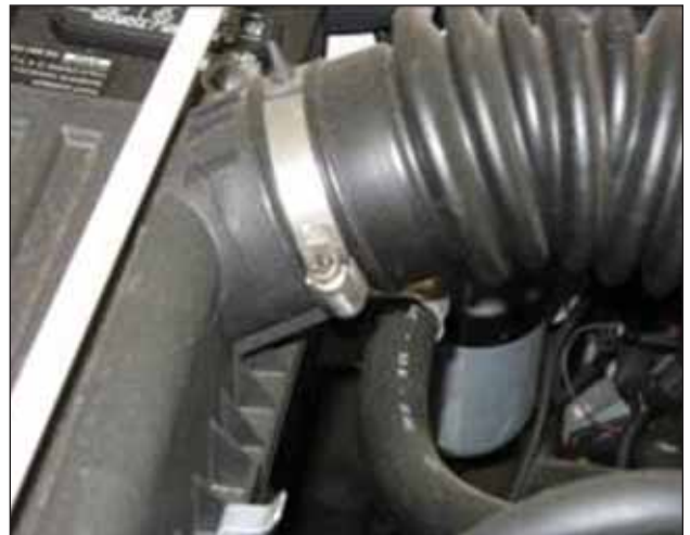
d. Loosen the hose clamp connecting the intake tube to the air filter lid.
