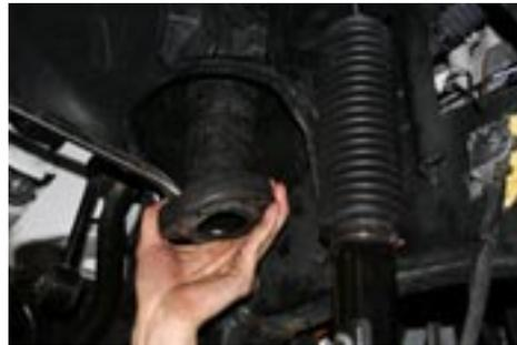
35. Install the new front spring spacer.
