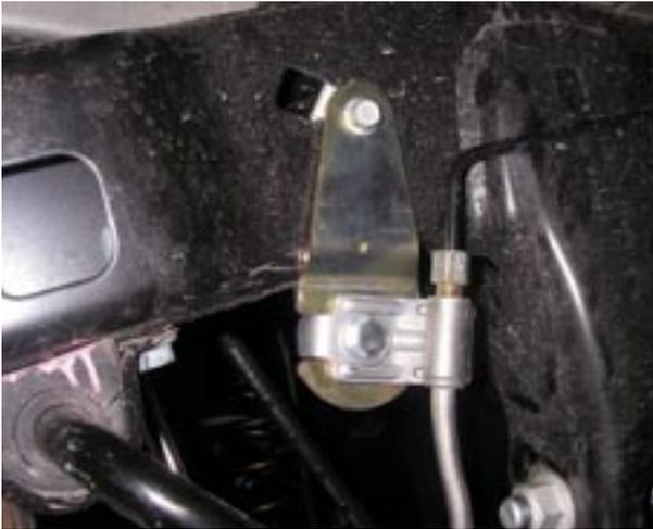
The rear brake line lowering brackets (**3-inch kit only. The 4-inch kit includes extended brake and L-Tabs to mount the lines to the frame**) are bent in order to allow additional clearance between the brake line and the rear factory sway bar. Be sure to install the left and right brackets so the brake line is moved in away from the sway bar. The locating tab should be located in the slot on the bracket.
