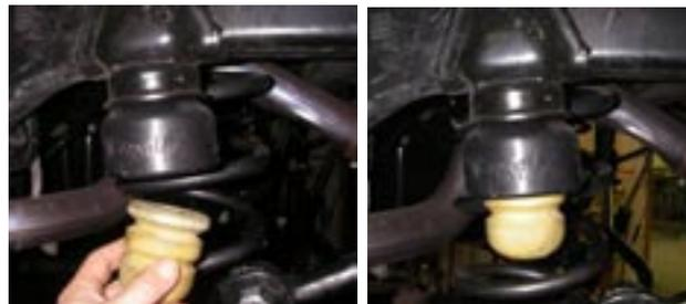
18. Install the lower bump stop onto the axle pad with the 5/16 x 1.25 bolts, washers and nuts provided in the hardware kit. **Note:** Make sure the bumpstop location is the same as photographed with the extra lip facing the front of the vehicle.
