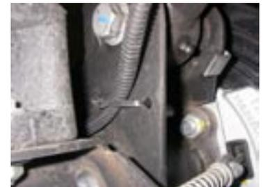
6. Replace the rear factory brake hoses with the new longer brake hoses.
