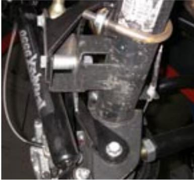
22. Raise the rear axle far enough to connect the track bar to the new bracket, using the factory bolt and nut.
