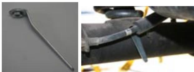
Insert the bolt, with the lockwasher on top of the flat plate, into the rear lower spring retainer, holding the flanged nut in place using the provided wrench tool and begin tightening the bolt. Remove the tool when finished.
