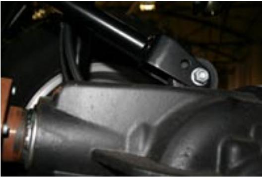
Note: Install the front upper arms as shown in the photo. **To avoid removing the exhaust, cut the right front upper control arm bolt on the frame end. A new bolt and nut are included in the kit. Install the new bolt from the outside in.** Each lower front FlexArm has a sticker to show where and how to install the arm. Make sure the sticker is up when the arm is installed.
