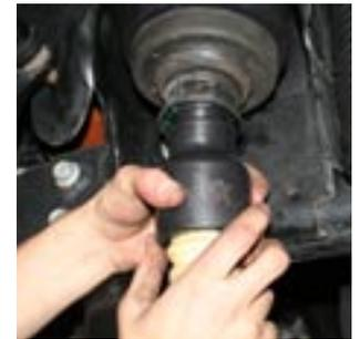
39. Set the length of the front upper FlexArms to 19-1/2". Final length adjustment will happen during the alignment.
